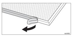
Before using the appliance take out the grease filter and remove the protective foil from the filter frame. Return filter.
